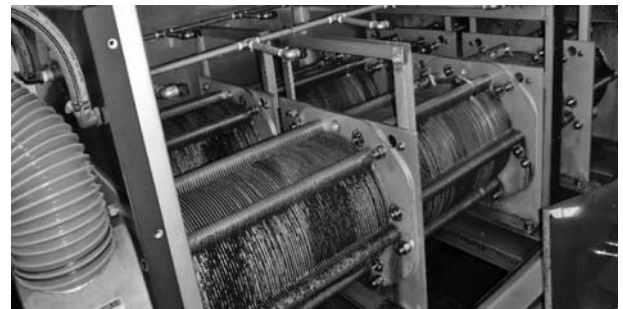
Photo. 6 Dewatering Unit Field Test for Optimization of Coagulant Dosing Rate and Solution Density
