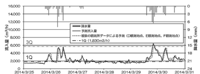
Fig. 4 Temporal change of inflow sewage water amount prediction by deep learning using 3 weather stations data
