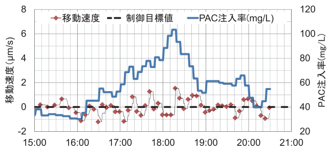
Fig. 12 Electrophoresis movement speed and coagulant dose rate during high turbidity raw water test
