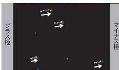
Fig. 4 An example of image processing in microscopic electrophoresis at high coagulant dose condition
