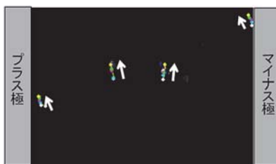
Fig. 3 An example of image processing in microscopic electrophoresis at appropriate coagulant dose condition
