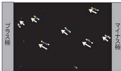
Fig. 2 An example of image processing in microscopic electrophoresis at low coagulant dose condition
