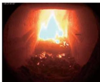
Fig. 1a Insufficient supply of waste
