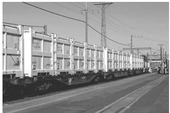
Fig. 6 The exclusive freight train for transporting waste 9)
