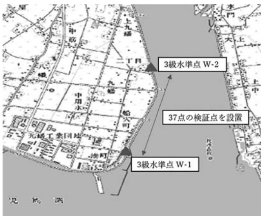
Fig. 5 Locations where the control points were set for accuracy verification
