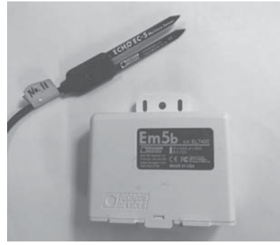
Fig. 1 Size of EC-5 Soil Moisture Sensor (Left), Picture of EC-5 Soil Moisture Sensor, Em5b Data Logger (Right)
