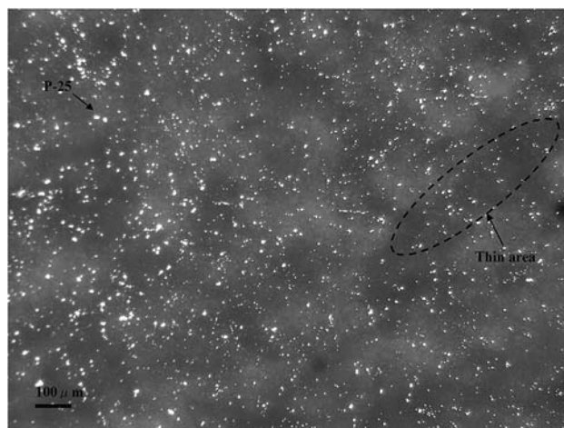
Fig. 2 Microscope picture of TiO 2 -coated responsive glass fundamental properties of the self-cleaning pH electrodes.
