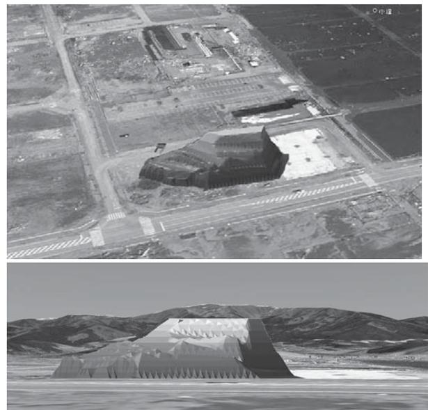
Picture.3: 3-Dimensional Contour Picture Re-Constructed of Actual Rubble Knoll in Rikuzen Takada City.
