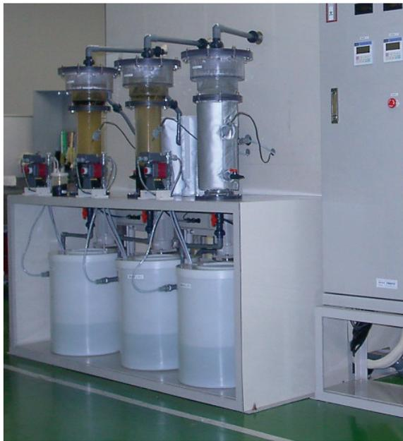
Photo.1: Lab scale anaerobic digestion treatment units
