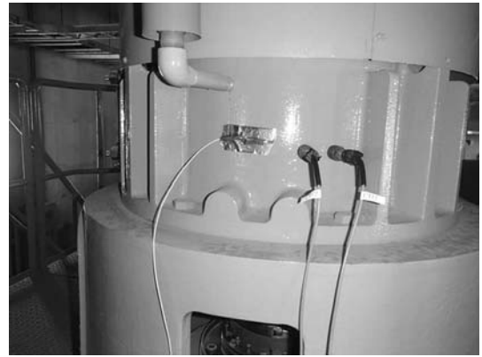
Photo 2 Vibration galvanometer, the sound-level meter setting situation
