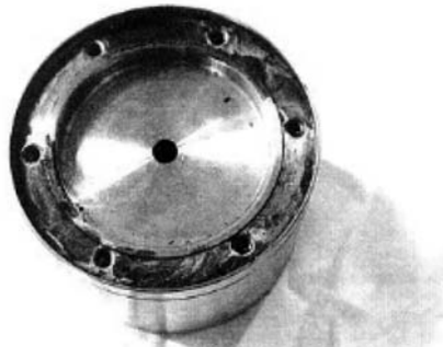
Photo. 1 The unit body corrosion situation for the protection
