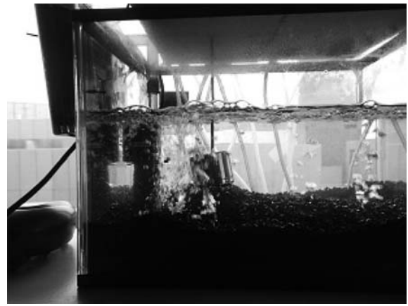
Photo. 5 Corrosion experiment scenery with the simulated bio film filtration pond
