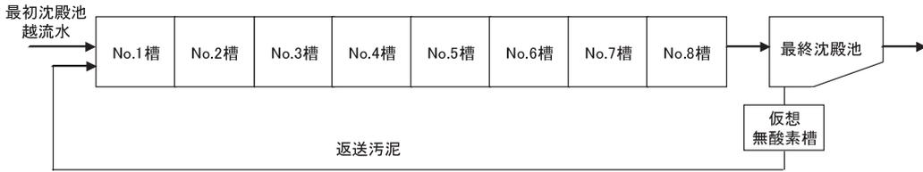
Fig. 2 Flow diagram (ASM)
