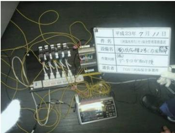
Photo. 4.2 Investigation. Setting of data logger and AC-DC converter.
