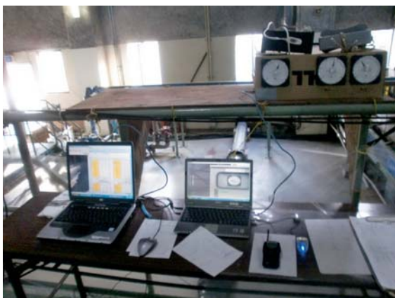
Photo. 1 A temporary monitoring control system of dehydrator which consists of a notebook PC and instrumentation attached to card box. (Date Taken : October 2011 at Sen-En STP)
